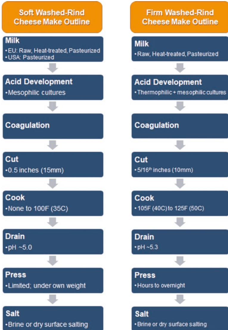
Fig. 19.1 General manufacturing steps and make procedure outlines for soft (left) and firm/hard (right) washed-rind cheeses (Provided by author)
