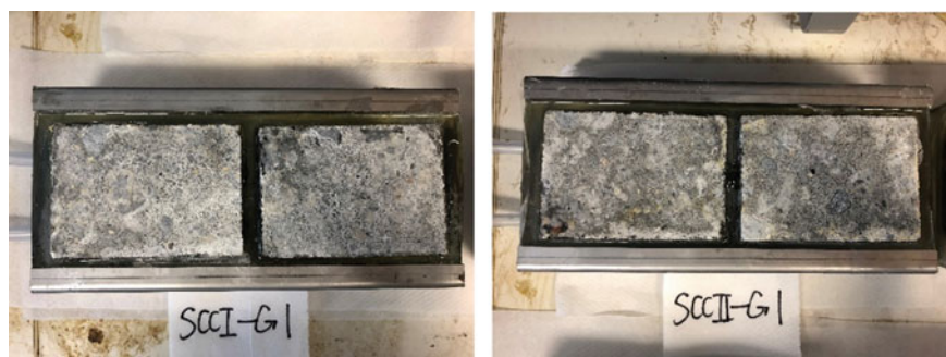
Fig. 8 Photos of the embedded concrete coupons of two concrete products, i.e. SCC-I and SCC-II
