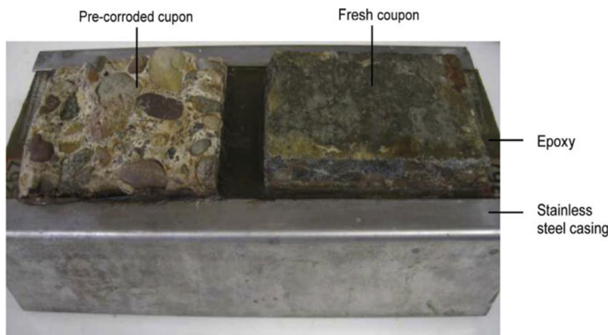
Fig. 1 Top front view of the mounting coupons in a stainless-steel casing. Reproduced from Sun et al. [24] with permission from Elsevier
