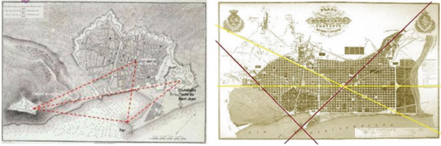
Fig. 11.3 The triangle measured at Barcelona, and the position of meridian and parallel
