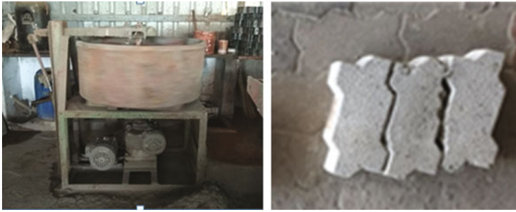
Fig. 15.3 Paver blocks preparation
