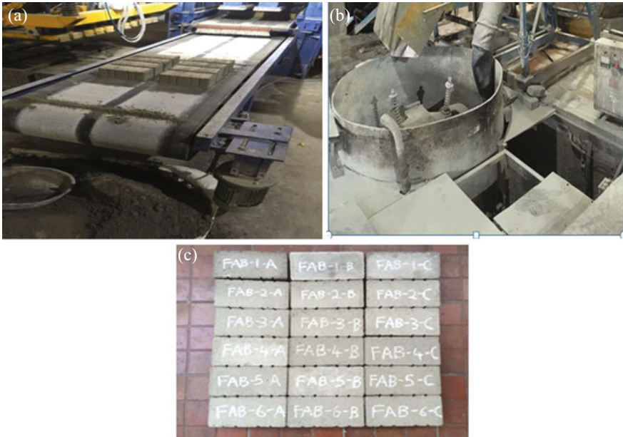
Fig. 17.3 Flyash bricks preparation a Mixing of raw materials b Bricks emerging from hydraulic press c Bricks after curing
