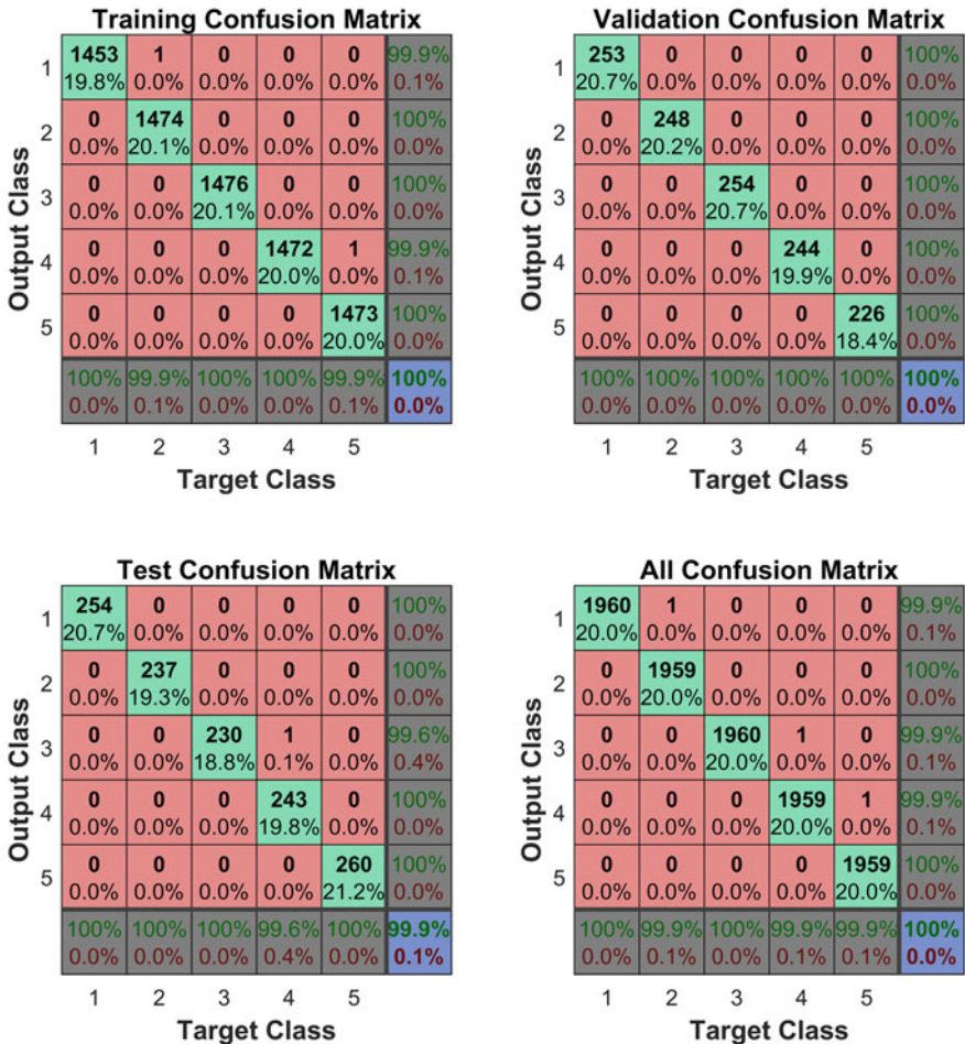
Fig. 17 MW power MDNN’s confusion matrix showing accuracy of training
