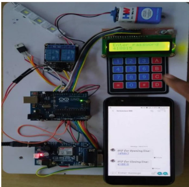
Fig. 9 Line in open (Hardware) with OTP message
