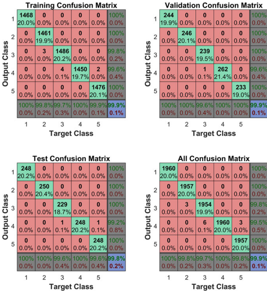
Fig. 22 MVAR power MDNN’s confusion matrix showing accuracy of training
