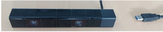
Fig. 3. The used stereo camera is a Sony PlayStation 4 camera model 1. The camera provides two 1280 \times 800 images. The cable was modified to be used on a standard USB3 port.
