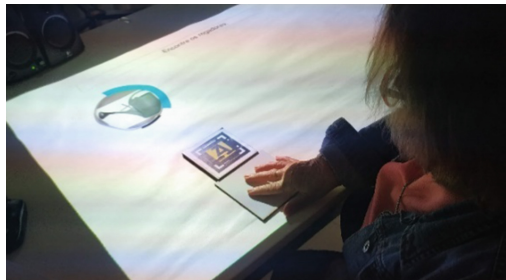
Fig. 4. Participant manipulating a physical object with a marker that controls the virtual cursor. The activation of the 4-s timer when selecting an answer.
