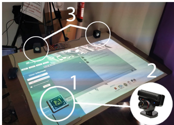
Fig. 1. Projection-based augmented reality system. 1) Physical object with a marker attached to it. 2) PSEye camera attached to the projector to track the position of the physical objects. 3) External speakers for the music and feedback. The table was covered with a white sheet of paper to enhance the contrast of the virtual projection.
