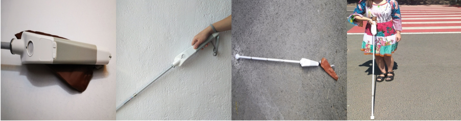
Fig. 1. The WeWALK design. The leather pouch is used to protect the sensors from extreme environmental conditions. The sensors in the handle will vibrate when there are some obstacles nearby. The participant needs to swipe the smart cane to identify the obstacles along the path.
