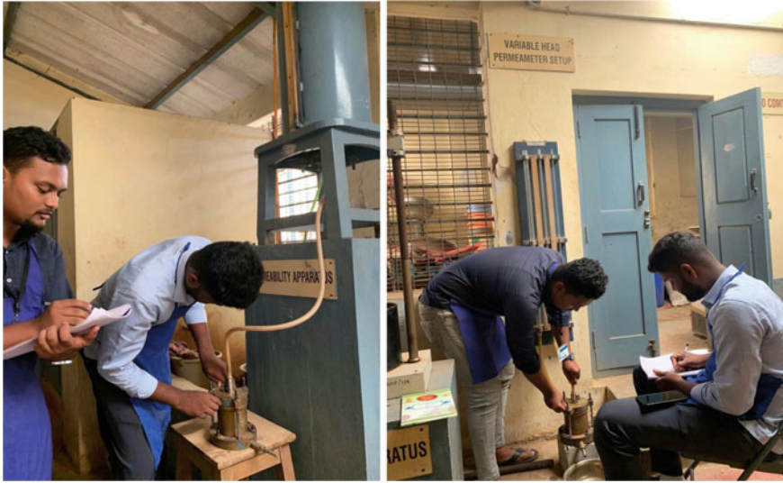
Fig. 5 Saturated hydraulic conductivity tests at laboratory
