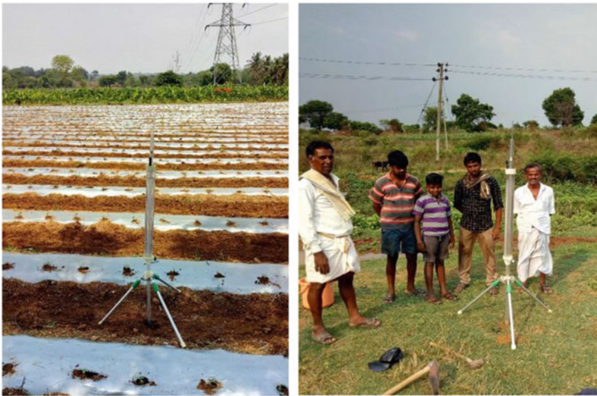
Fig. 4 Guelph permeameter at site
