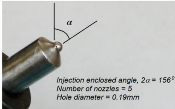
tip. After start of injection (SOI), the fuel spray was observed for a duration of up to 5 ms as further time would result the spray to reach to the wall of the cylinder. After that, the images were transferred to the i-SPEED Viewer software, and the spray measurements were performed using the SolidWorks CAD software. This technique was also described in the previous study in determining the spray characteristics by visualization (Soid and Zainal 2014).
