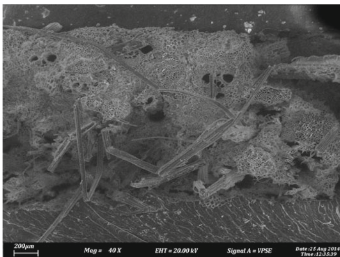
Fig. 2.8 Failure modes of laminated strip bamboo
