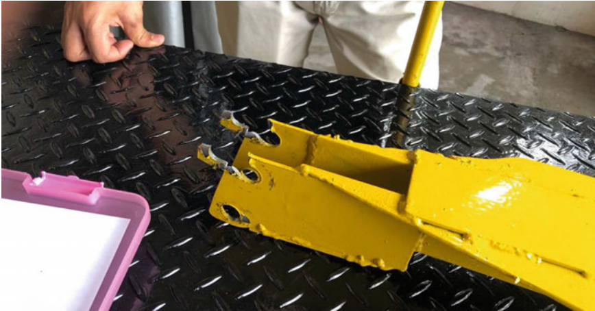
Fig. 11.2 Failure at hydraulic arm
