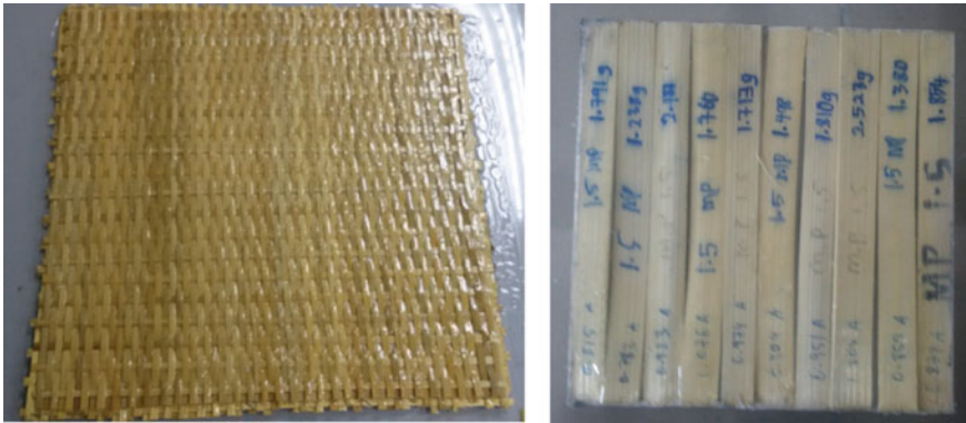
Fig. 2.1 Laminates of woven and strip bamboo
