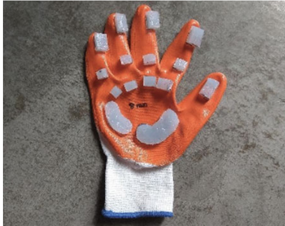
Fig. 19.7 Inner condition of the dampening glove with silicone rubber
