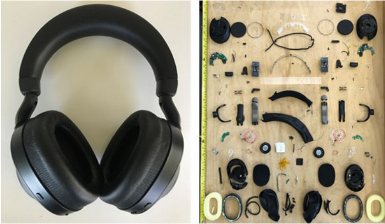
Fig. 2.3 Headphone Jabra Evolve2 85 before (left) and after dismantling (right)
