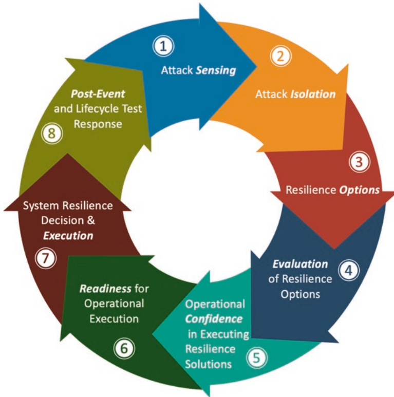
Fig. 21.10 Overview of the Framework for Operational Resilience in Engineering and Systems Test (FOREST)
