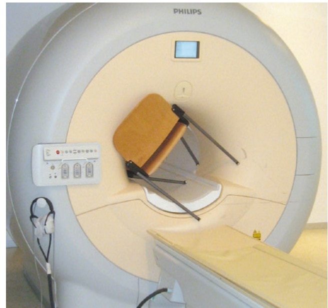
Fig. 2.1 The main magnetic field will attract any ferromagnetic devices converting them into dangerous projectiles
