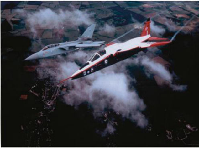
Fig. 3.14 Negative tailplane lift on Tornado. Positive tailplane lift on FBW Jaguar. (Photograph by Arthur Gibson provided by British Aerospace Defence Ltd.)
