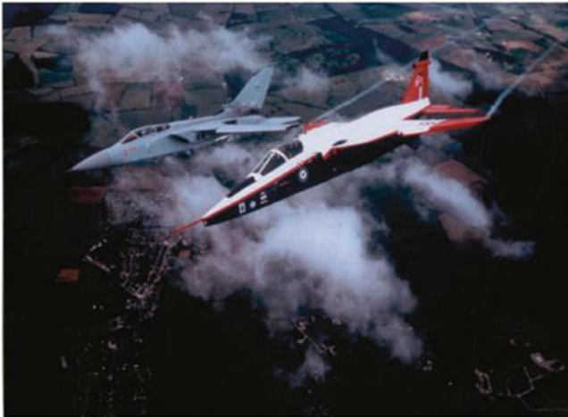
Fig. 3.14 Negative tailplane lift on Tornado. Positive tailplane lift on FBW Jaguar. (Photograph by Arthur Gibson provided by British Aerospace Defence Ltd.)
