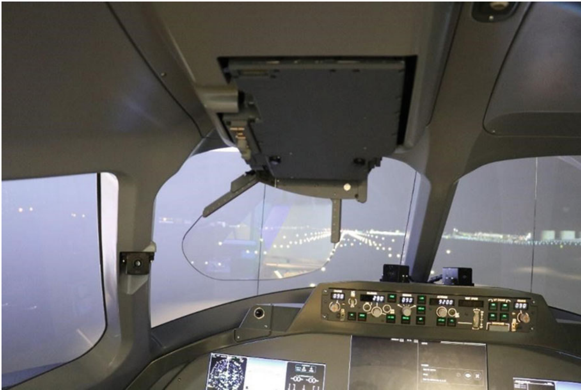
Fig. 2.52 LiteWave® overhead HUD. (Courtesy of BAE Systems)
