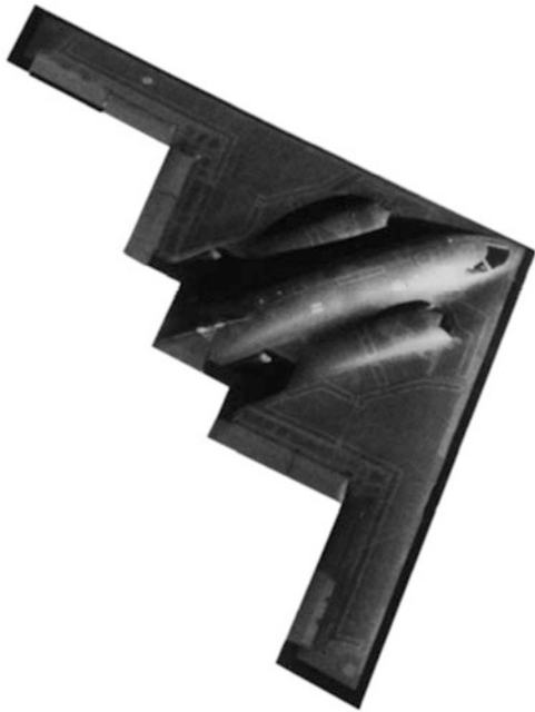
Fig. 4.10 Northrop B2 ‘Spirit’ strategic bomber. (Courtesy of the Royal Aeronautical Society Library). Note ‘flying wing’ configuration and absence of vertical surfaces; yaw control being achieved by the operation of split ailerons
