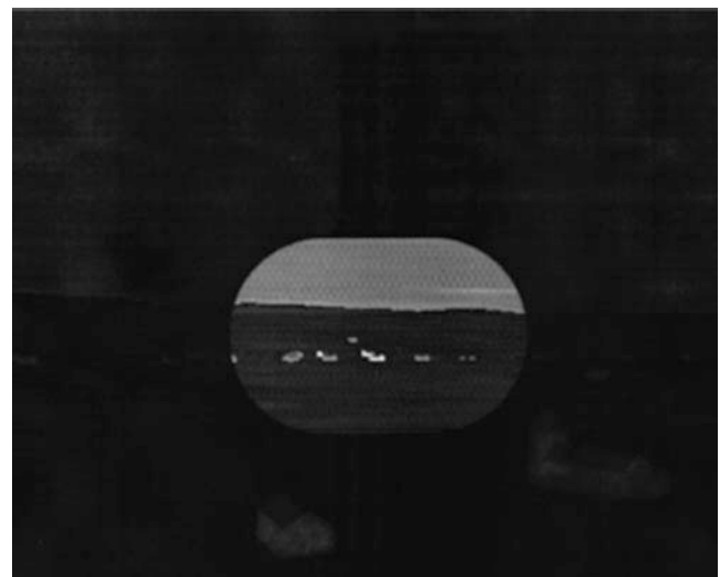
Fig. 2.10 Instantaneous FOV of conventional HUD
