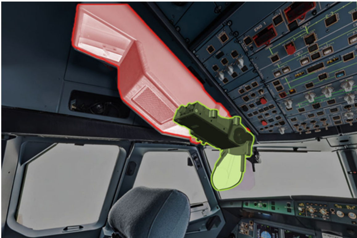
Fig. 2.53 LiteWave® is considerably smaller than existing conventional HUDs. (Courtesy of BAE Systems)
