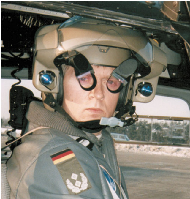
Fig. 2.29 Helicopter HMD with integrated NVGs (Courtesy of BAE Systems). This HMD forms part of the mission systems avionics for the Tiger 2 attack helicopter for the German army
