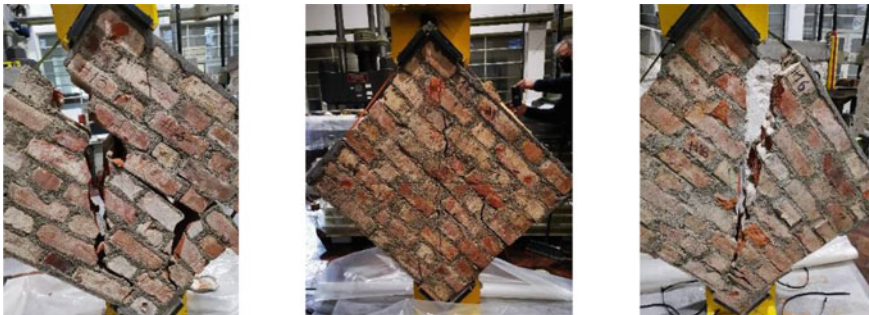
Fig. 7 Rupture mode of 1:5 cement-sand mortar wallettes
