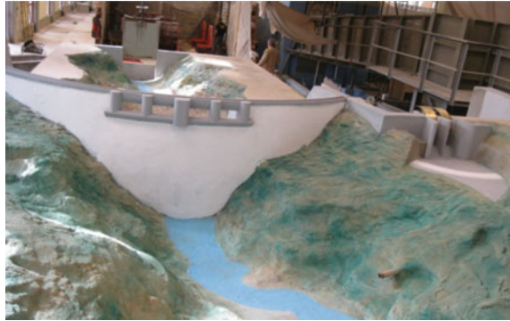
Fig. 2 Physical model of Salomonde Dam built using the traditional method, [1]
