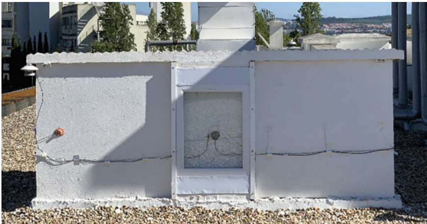
Fig. 4 Photo of the test cell built to study the thermal behaviour of the SBRS
