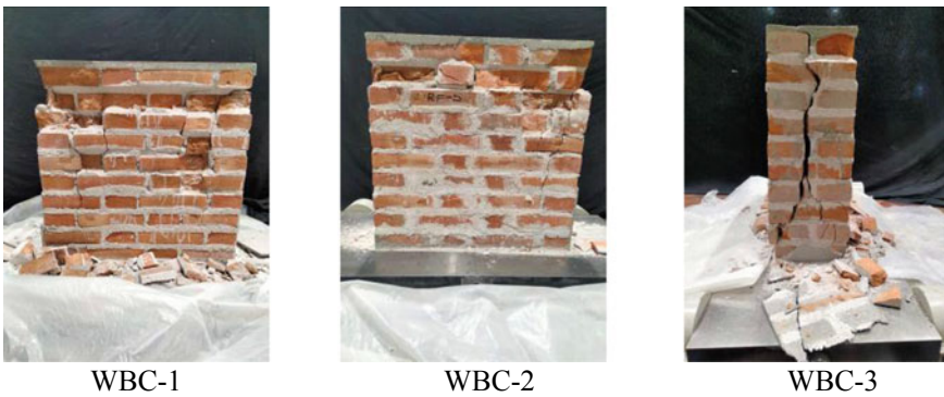
Fig. 10 Compressive rupture mode of 1:3:12 cement-lime-sand mortar wallettes
