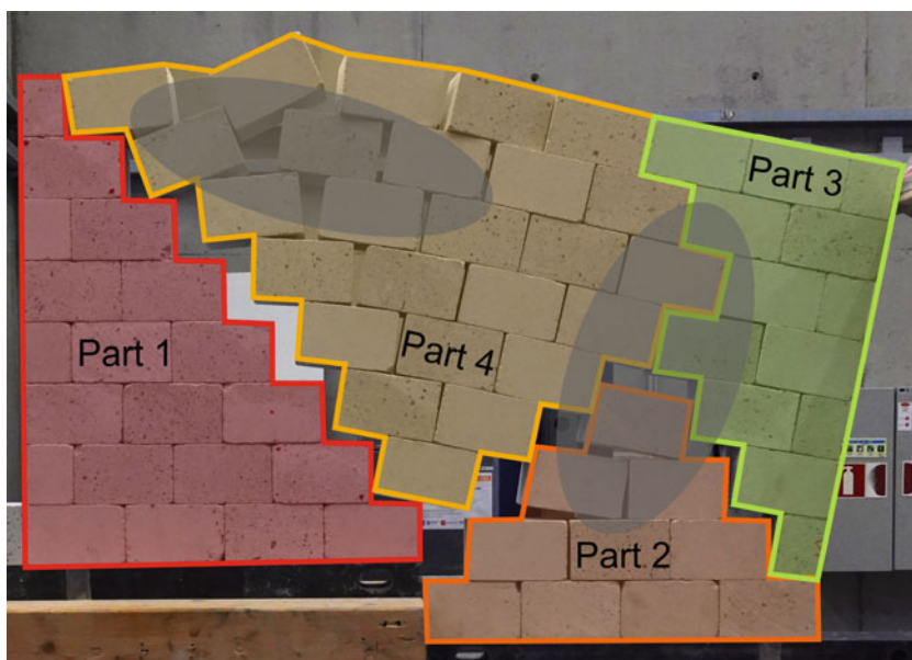
Fig. 10 Representative collapse mechanism obtained at the end of the settlement on the third configuration. Similar mechanisms are observable for the second and the fourth configurations. The shear wall is divided into four parts with frictional dissipations between them
