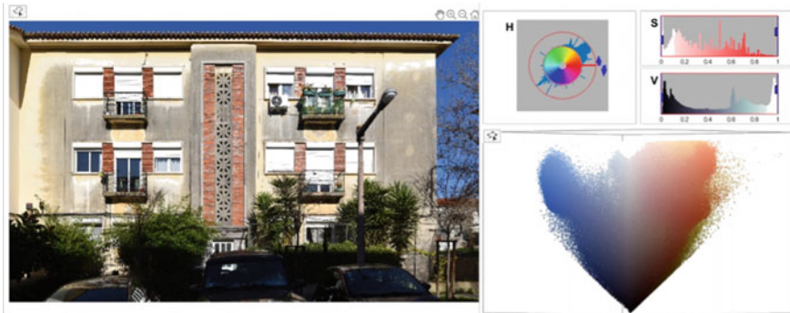
Fig. 4 Visualization of the colour thresholder (example of façade No.4)
