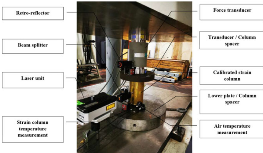
Fig. 2 Experimental apparatus for the strain column calibration
