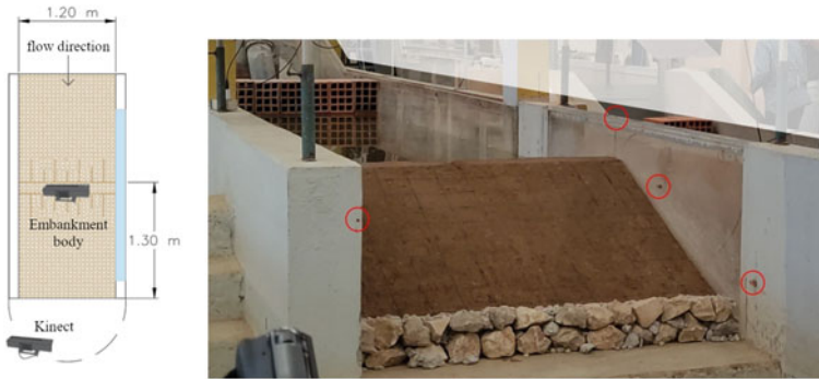
Fig. 11 Layout adopted for the Kinect Sensor during testing and location of targets of known coordinates for the characterization of the 3D dam morphology during the failure
