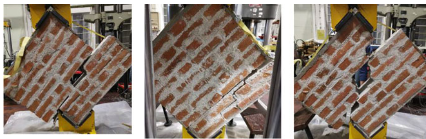
Fig. 8 Rupture mode of 1:3:12 cement-lime-sand mortar wallettes
