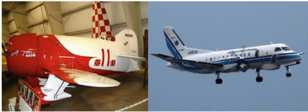
Fig. 1. The effect of specific. The Gee Bee racer from 1932 (left) with a piston engine with 1.2 kW/kg, where the engine is about half of the empty weight of the aircraft, and the Saab 340 (right) with turbo shaft engines with about 8 kW/kg. Both have a comparable top speed of 476 km/h and 502 km/h respectively.
