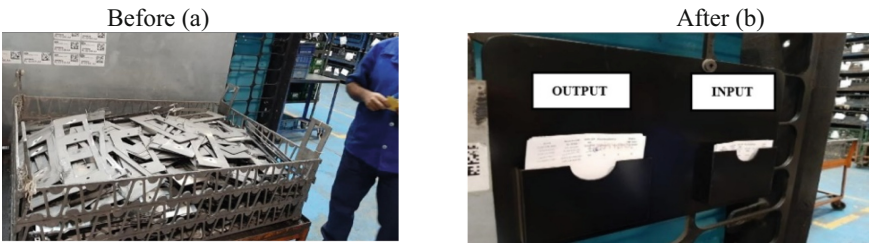
Fig. 4. (a) and (b). Cardboard for Input and Output Kit Assembly. (Source: Authors, 2022).
