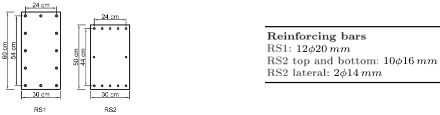
Fig. 6 RC sections: geometry and materials
