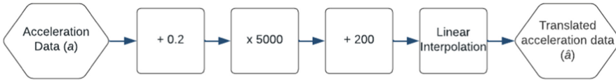
Fig. 5. Process used for the translation of the footbridge acceleration data to the human audible range.
