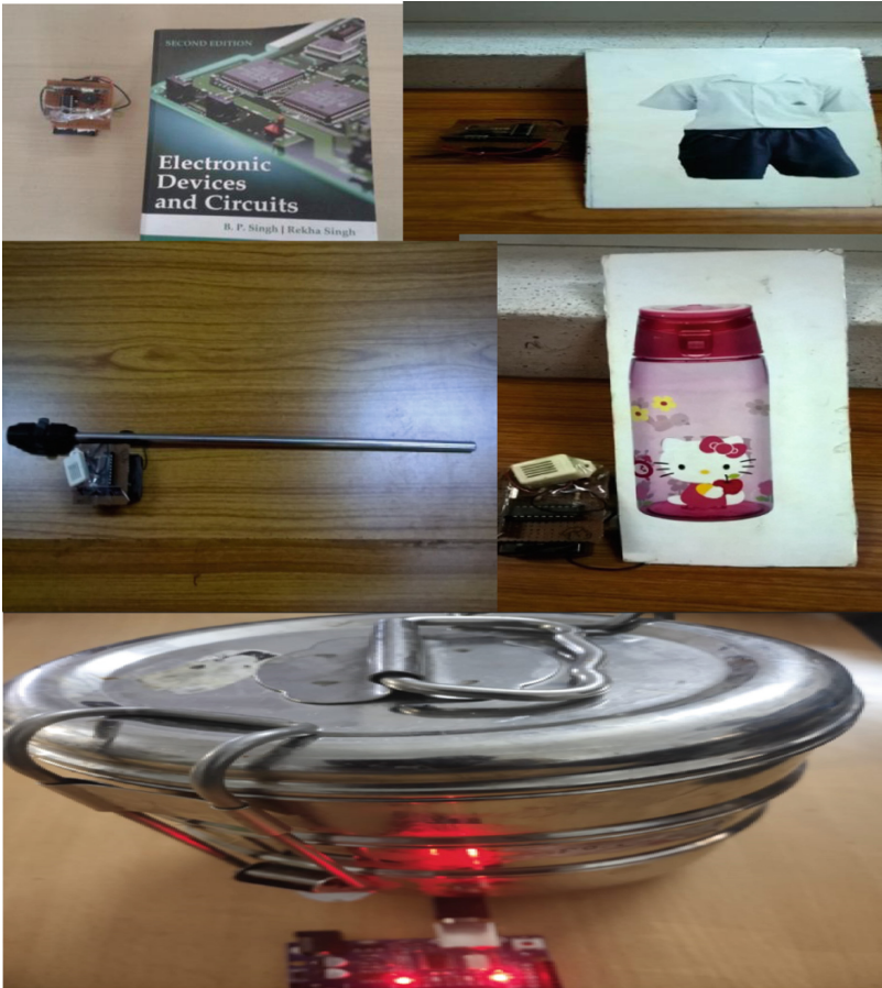
Fig. 8. RFID Tags attached to the different objects (Bottle, Lunch Box, Uniform, Stick, Book)
