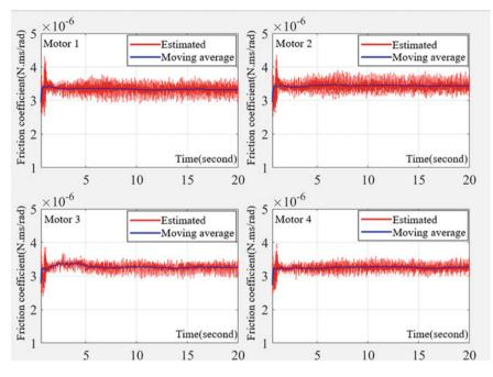
Fig. 12 Friction coefficient of motors during PMD hovering
