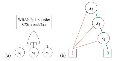
**Fig. 6** Reliability models for evaluating P(WBAN fails| $IE_{1,1} \cap CRE_{1,I}$ ). **a** Reduced DFT, **b** BDD
