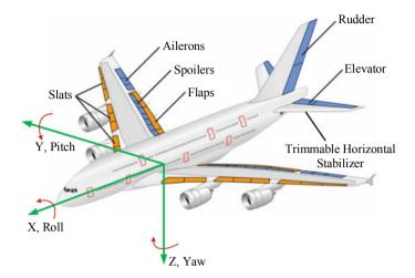
Fig. 1 Control surfaces of an advanced commercial aircraft
