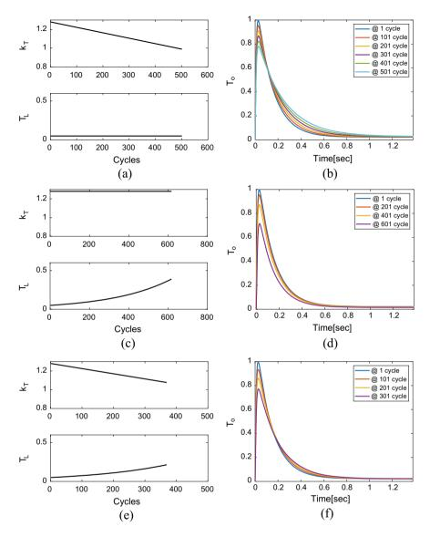
Fig. 5 Output torque due to components degradation, **a** health parameters and **b** output torque of case 1, **c** health parameters and **d** output torque of Case 2, and **e** health parameters and **f** output torque of Case 3
