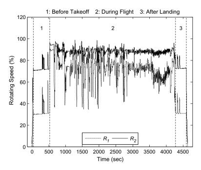
Fig. 3 The two rotating speeds of a typical sortie
