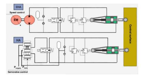
Fig. 6 HA/EHA heterogeneous actuation system
