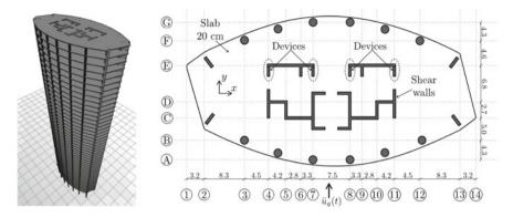
Fig. 6 Isometric view (left) and floor plan (right) of the 52-story building model. Example 2
