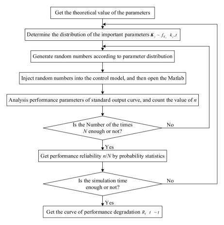
Fig. 17 Reliability simulation flow chart
