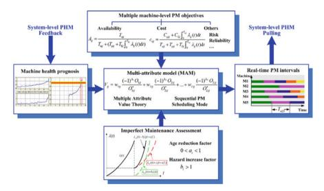
Fig. 2 Illustration of machine-level MAM method
