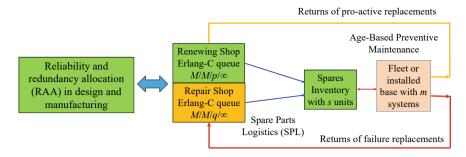
Fig. 2 Single echelon supply chain for system availability support
