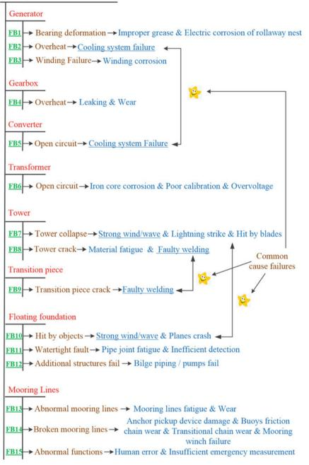
Fig. 5 Failure behaviours of FOWTs [8]
