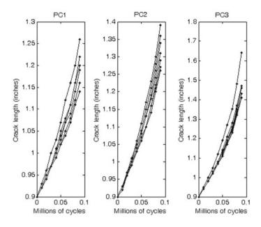
Fig. 5 The development of crack sizes over time
