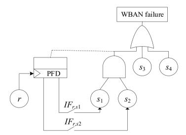
Fig. 4 Fault tree of the example WBAN system
