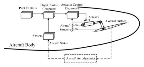
Fig. 2 Aircraft flight control system
