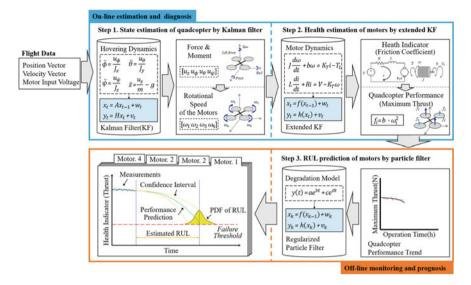
Fig. 11 The Quadcopter PHM framework
