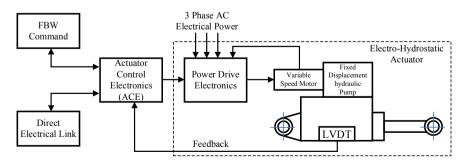
Fig. 5 Electro-hydrostatic actuator (EHA)
