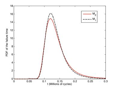
Fig. 2 PDFs of the failure time based on model  $M_1$  and  $M_2$  (fatigue cracks)
