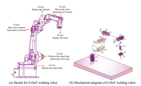
Fig. 2 A 6-DoF welding robot
