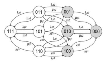
Fig. 6 CTMC of processor subsystem
