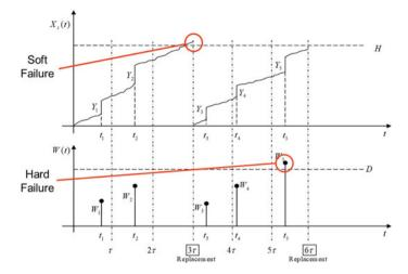
Fig. 7 Two dependent competing failure processes: soft failure process and hard failure process
