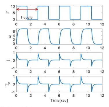
Fig. 4 Simulation result of DC motor system
