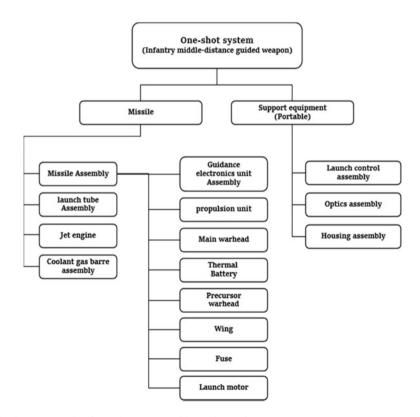
Fig. 1 An example of one shot system with regular equipment
