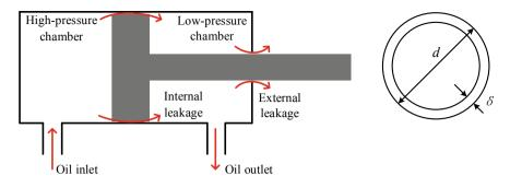
Fig. 15 The leakage diagram of a cylinder
