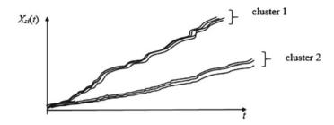
Fig. 10 Two clusters of degradation paths for seven identical components in a system [99]
