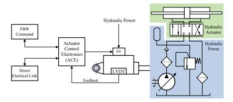
Fig. 3 Hydraulic actuation system
