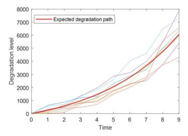
Fig. 4 Example of a non-linear gamma process
