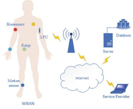
Fig. 1 Structure of a typical WBAN system
