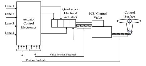
Fig. 4 Quadruplex actuation system
