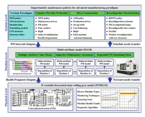
Fig. 1 Scheme of hierarchical PHM decision-making for CPS
