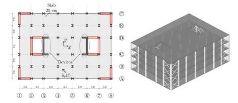
Fig. 9 Floor plan (left) and isometric view (right) of the 4-story building. Example 3
