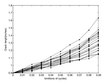
Fig. 1 The measurements of crack length over time
