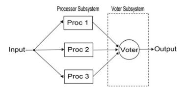
Fig. 4 Block diagram for TMR system with a voter
