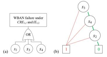
Fig. 7 Reliability models for evaluating P(WBAN fails| $IE_{1,2} \cap CRE_{1,I}$ ). a Reduced DFT, b BDD
