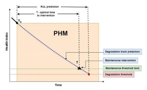
Fig. 1 PHM-based RUL prediction and optimal maintenance action scheduling
