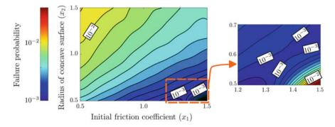
Fig. 3 Iso-probability curves in the design space. Example 1
