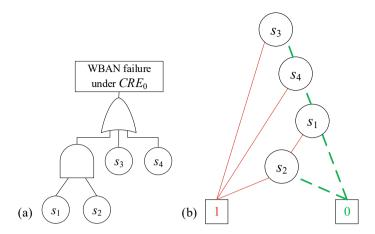
Fig. 5 Reliability models for evaluating  $W_0$ . a Reduced fault tree and b BDD
