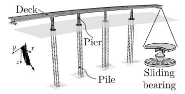
Fig. 1 Isometric view of the nonlinear bridge model. Example 1
