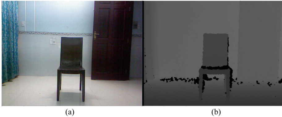
Fig. 5. Example of depth map obtained from Kinect, (a) practical image, (b) depth map.
