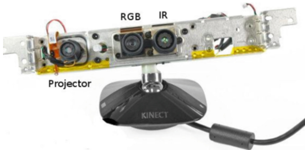
Fig. 1. Inside structure of Kinect camera.
