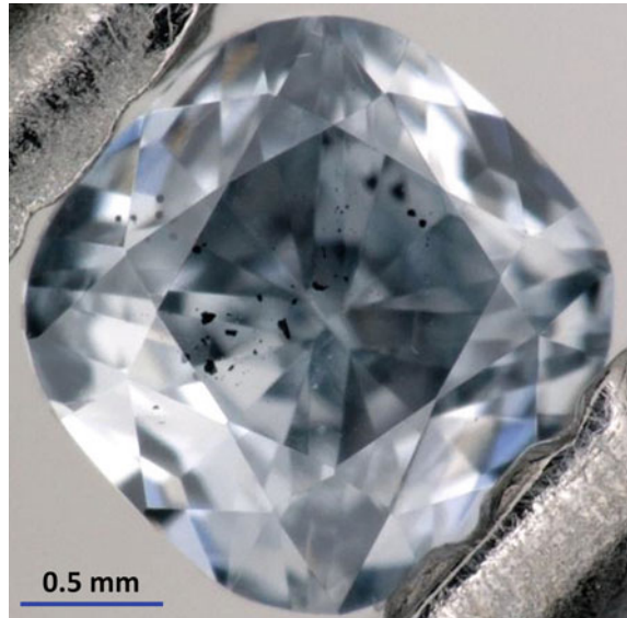
Fig. 10.6 Ferropiclasite inclusions (50–100 \mu\text{m} black minerals) in blue, super-deep diamonds (Smith et al. 2018). Photo by Evan Smith, GIA
