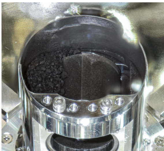
Fig. 11.5 Ryugu particles collected during the first touchdown operation. The diameter of the sample canister is 48 mm (Sawada et al. 2017)
