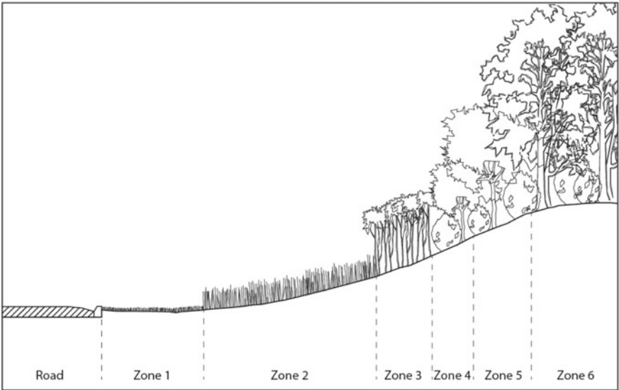
Fig. 2.5 Section across a grid road verge showing the zonal structure. Source Kelcey and MKDC (1974)
