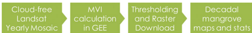
Fig. 12.1 Summary of the workflow for generating the decadal mangrove maps and statistics. More detailed information on MVI-based mapping was described in Baloloy et al. (2020). Here, the MVI was first applied to Sentinel-2 imageries to map the 2019 mangrove extent in the Philippines
