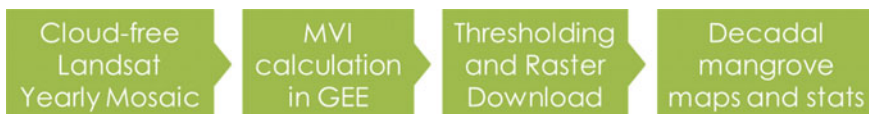
Fig. 12.1 Summary of the workflow for generating the decadal mangrove maps and statistics. More detailed information on MVI-based mapping was described in Baloloy et al. (2020). Here, the MVI was first applied to Sentinel-2 imageries to map the 2019 mangrove extent in the Philippines
