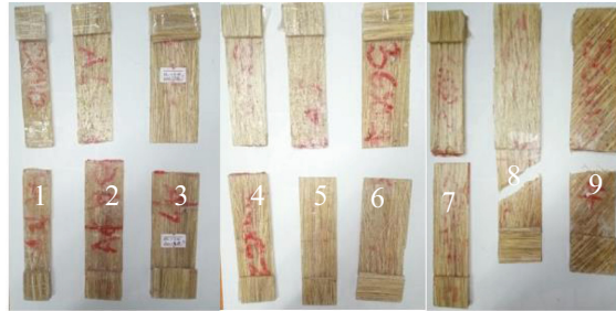
Fig. 9. Failure mechanism of adhesive joined DPFRPC
