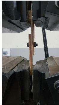
Fig. 4. Tensile test of single lap bolt joint DPFRPC using UTM: WAW-600D
