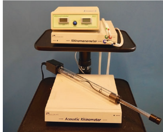
Fig. 13.4 Combination of 3 electronic instruments for assessing nasal obstruction. Rhinospirometer (top), Rhinomanometer (middle), and Acoustic rhinometer with sonic tube (bottom)
