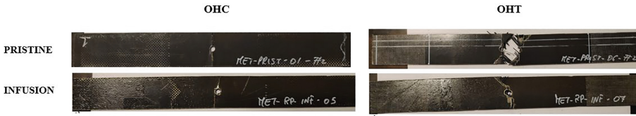
Fig. 2. Failure mode OHC and OHT tests
