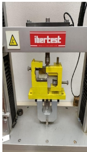
Fig. 4. Iosipescu test device view
