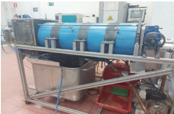
Fig. 1. Slamming Playback Equipment with built-in eccentric cam
