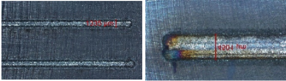
Fig. 12. Microscope acquisitions of the new deposited layers and bead width.
