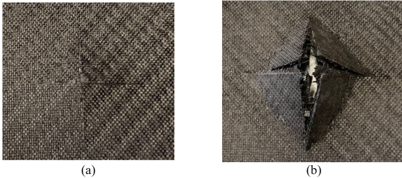
Fig. 7. Composite plates after the impact tests: a) impact energy of 15 J; b) impact energy of 30 J.
