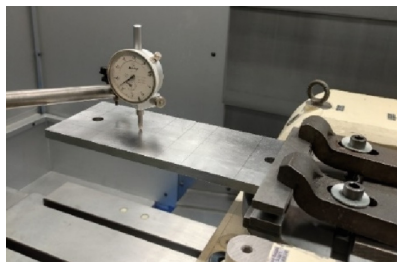
Fig. 9. Comparator setup with the clamped substrate.
