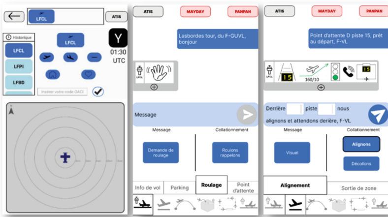
Fig. 3. MSCD tablet interface (left) ATIS application, (middle) taxiing interface, (right) alignment on the runway
