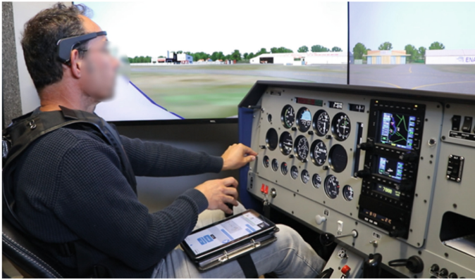
Fig. 2. Pilot in the flight simulator with the MSCD (tablet attached to the knee and haptic vest) and EEG used for experimental studies
