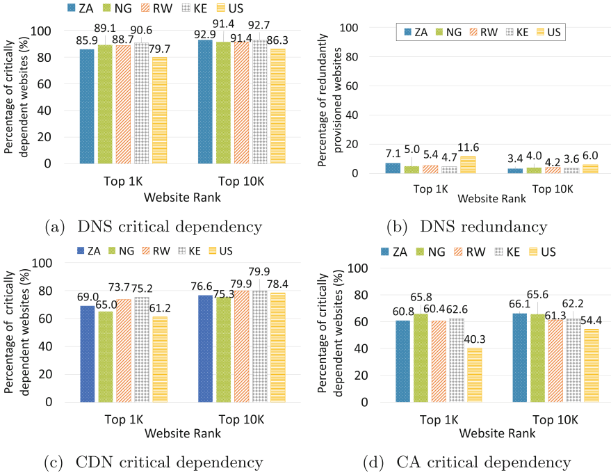
Fig. 3. (a) Critical DNS dependency for top 10K US-visited sites when measured from a US vantage point is 5% to 7% less than the top 10K Africa-visited websites. This gap in critical dependency increases to 6% to 10% in the more popular (top 1K) websites. (b) The percentage of websites that are redundantly provisioned is slightly higher (2%) in the US-visited websites as compared to the Africa-visited websites. However, when we look at more popular websites (top 1K), for US-visited , the percentage of redundantly provisioned websites is 5% to 7% higher than the Africa-visited websites. (c) Critical CDN dependency for the top 10K US-visited sites is similar to the top 10K Africa-visited websites. However, for more popular websites, US-visited sites are 4% to 15% less critically dependent than Africa-visited sites. (d) Critical CA dependency for the top 10K US-visited sites, when measured from a US vantage point, is 7% to 12% less than the top 10K Africa-visited websites. This gap in critical dependency increases to 20% to 25% in the more popular (top 1K) websites.
