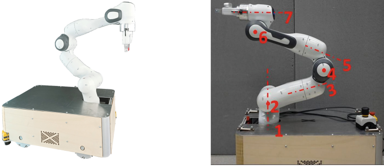
Fig. 1. Mobile manipulator LeoBot including the 7 rotational axis of the serial manipulator (red). (Color figure online)
