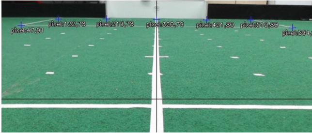
Fig. 3. With the camera mounted onto the robot, pixels corresponding to field points with known positions are hand-marked, for instance, penalty area corners, field corners, goal corners, or the goal center can be used. A PnP problem for the 2D points and their three-dimensional correspondences is solved by minimizing re-projection error. The employed algorithm is an implementation from OpenCV library and computes the camera's rotation and translation vectors with respect to field coordinates.
