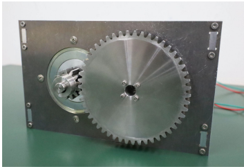
Fig. 4. Torque measurement device
