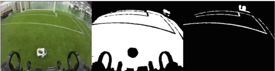
Fig. 11. Example of white line and green detection by deep learning (Color figure online)
