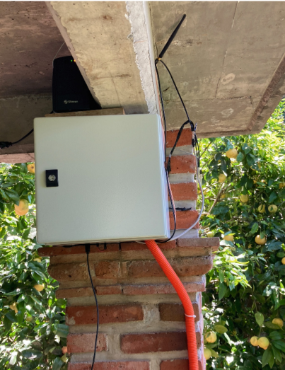
(c) Shield protection of the IoT device
