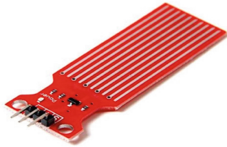
Fig. 7. Image of water level sensor
