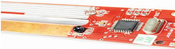
Fig. 4. Economic PH sensor with luminous intensity sensor.
