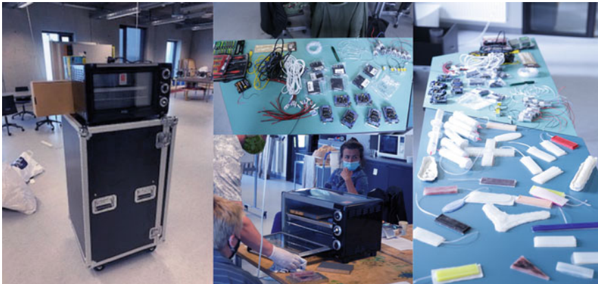
Fig. 13.1 Materials used for the soft robotics workshop. Left and center: electronics and oven used for curing silicone. Right: silicone actuators and pumps
