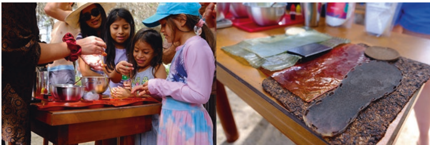
Fig. 30.3 Making bioplastics from agar, derived from algae (left), an array of bioplastics made from coffee waste, fish gelatine, tea waste and algae (right). (Photos: Jess Howard)
