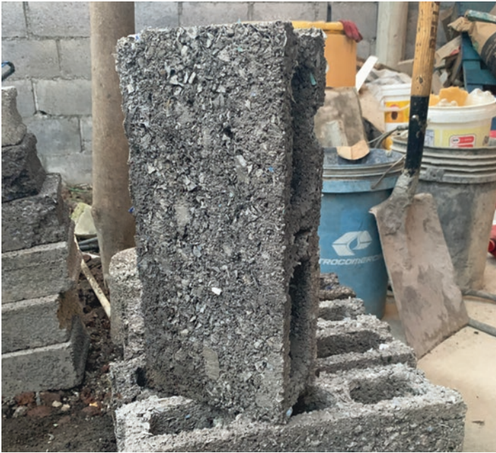
Fig. 30.2 Prototype plastic-enhanced concrete construction block, made from plastic collected from beaches in Galapagos. (Photo: Jess Howard)
