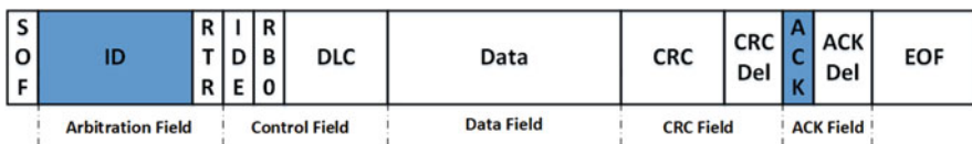
Fig. 4 The CAN data frame format
