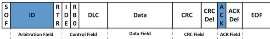
Fig. 4 The CAN data frame format
