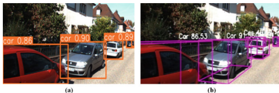
Fig. 5 Object detection modalities: (a) 2D vs. (b) 3D
