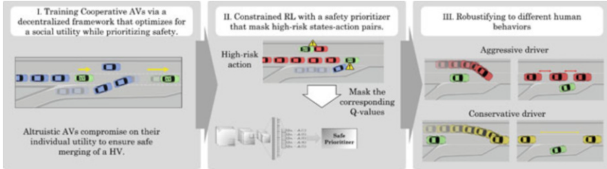
Fig. 4 An overview of our approach to leverage social awareness and coordination to improve the safety and reliability of CAVs. Our social-aware AVs learn from scratch not only to drive but also to understand the behavior of HVs and coordinate with them, they learn to adapt and influence HVs in a robust and safe manner
