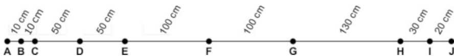
Fig. 9 Node positioning along the experimental bus model employed for evaluating TIDAL-CAN and CAN-SQUARE
