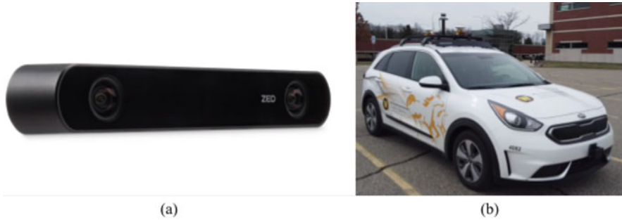
Fig. 2 (a) The ZED 2 camera sensor [22] and (b) The instrumented WMU EEAV lab research vehicles platform
