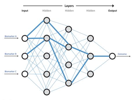
**Fig. 27.4** Deep learning showing the input, hidden, and output layers. In the example shown, line thickness between nodes in the various layers indicate biomarker features that have the greatest impact weight on the final output
