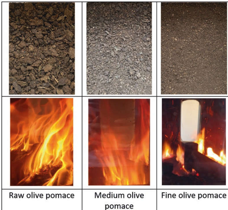
Fig. 12.4 Example of flames obtained according to the particle size of olive pomace
