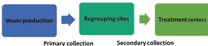
Fig. 1.5 Collection system steps
