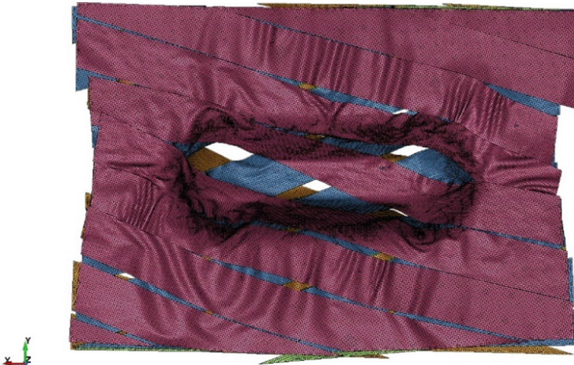
Fig. 9. Gap formation on angle-ply with 15°
