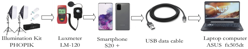
Fig. 3. Video signal acquisition system connection sequence.
