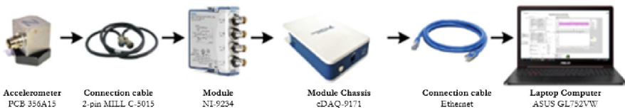
Fig. 2. Connection sequence of the vibration signal acquisition system [10].
