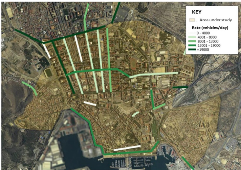
Fig. 2. Traffic map of the city, where the streets have been classified according to the ratio vehicles/day.
