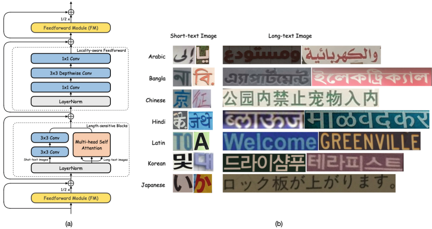
Fig. 3. (a) Architecture of Length-sensitive Encoder (LE). (b) Left: Examples of short-text images in each language. Right: Examples of long-text images in each language.
