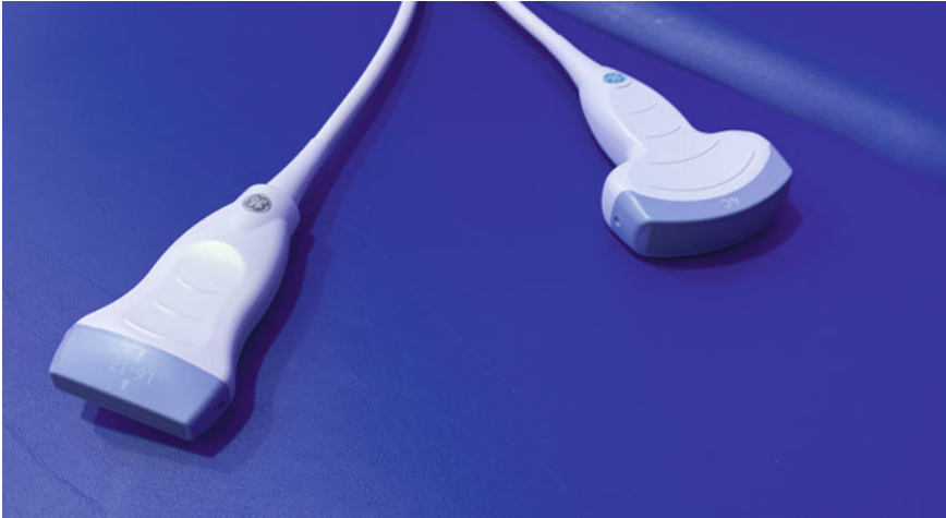
Fig. 3.2 On the left, a linear array probe, and on the right a curved array probe
