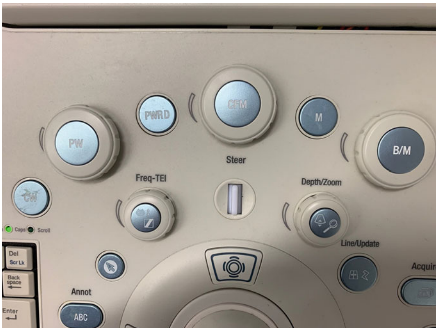
Fig. 2.2 The figure indicates three special knobs, the left one for changing the frequency, the right lower one for selecting the depth, and the right upper one (B/M) knob for adjusting the overall gain
