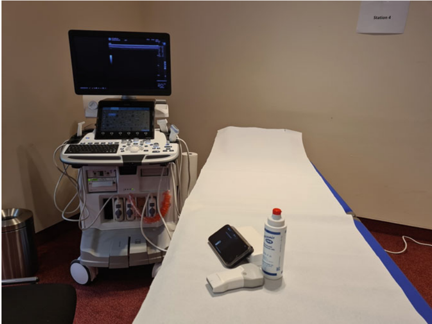
Fig. 3.1 An optimal combination of modern ultrasound machines. On the left, a high-end ultrasound system configured with several probes including a hockey stick, and on the right a handheld pocket-sized probe that includes a convex and linear array scanner and sends the information by Bluetooth to a mobile phone or tablet
