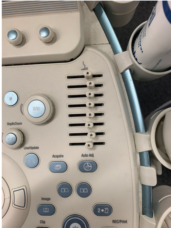
Fig. 2.1 This picture shows the line-up of 8 time gain control slides on the ultrasound machine. The topical hierarchy of the slides corresponds to the gain position on the ultrasound image, i.e., the upper slides control the gain for the upper part of the image, the lower slides for the lower (deeper) tissues on the ultrasound image
