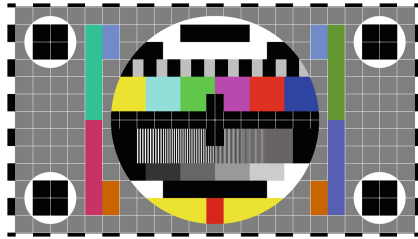
Fig. 8. Monoscope test pattern Philips PM5544
