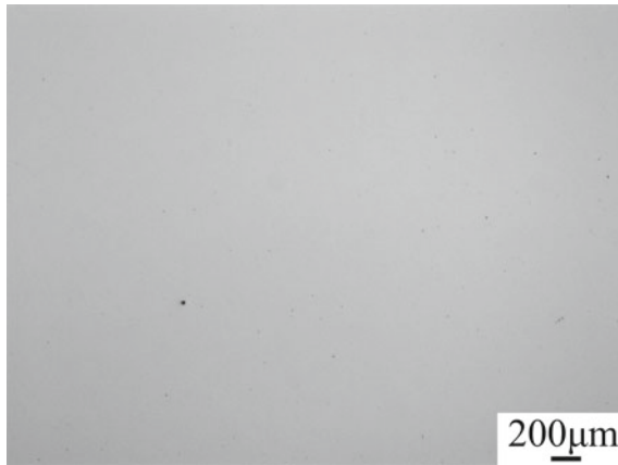
Fig. 8 Morphology of SLM-processed specimens at scanning power of 200 W and scanning speed of 1100 mm/s
