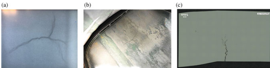
Fig. 10 ID crack in seam-welded pipe. a Radiograph, b ID view, and c Cross-section
