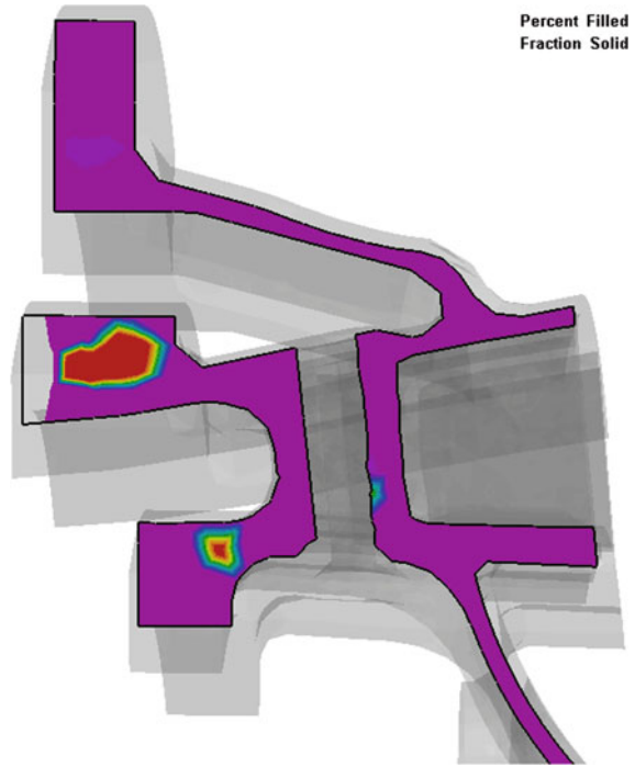
Fig. 9 Casting solidification prediction for an Alloy 718 component using a commercial casting solidification software showing hot-spot regions in locations where there is a propensity for solidification shrinkage porosity
