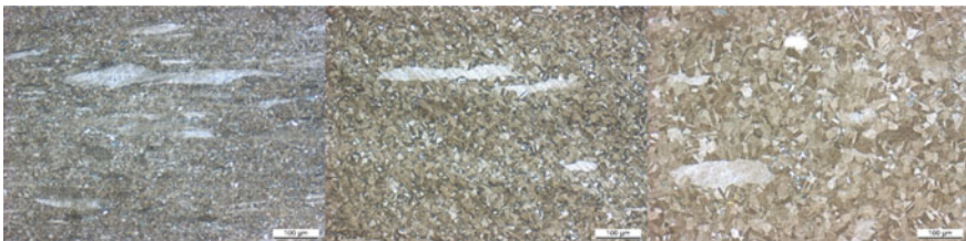
Fig. 7 Optical microscope images showing the grain structure for VDM 780 after Condition 2 (left), 3 (middle) and 4 (right). The forging direction is vertical. Samples were etched with 60 ml HCl (37%) and 10 ml HNO 3 (65%)
