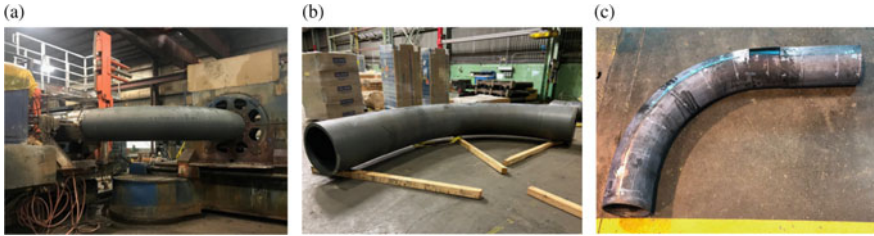
Fig. 5 Completed pipe bends. a Header pipe, b Reheater pipe, and c Welded pipe
