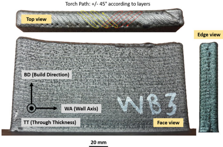
Fig. 1 Photograph of an IN718 LMD-w process wall labelled with axis directions
