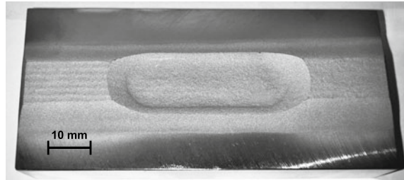
Fig. 4 Specimen in the as-sprayed condition. The image shows the sample Parameter II, according to Table 1. The surplus material is a result of the used spraying trajectory
