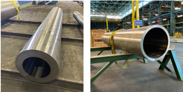
Fig. 3 Pipes prior to bending. Header pipe on left, reheater pipe on right
