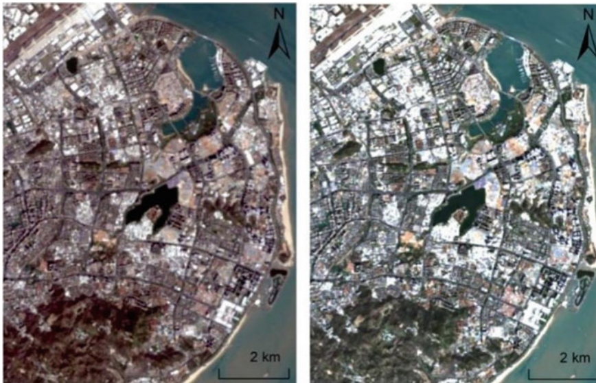
Fig. 1.3 Comparison chart before and after FLAASH atmospheric correction model (left: before atmospheric correction; right: after atmospheric correction)
