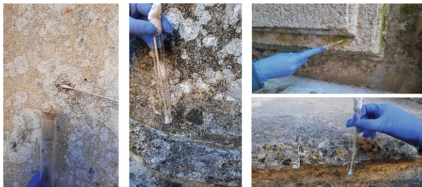
Fig. 10.2 Sample collection from various pigmented biofilms formed on the limestone walls of the Main Cloister
