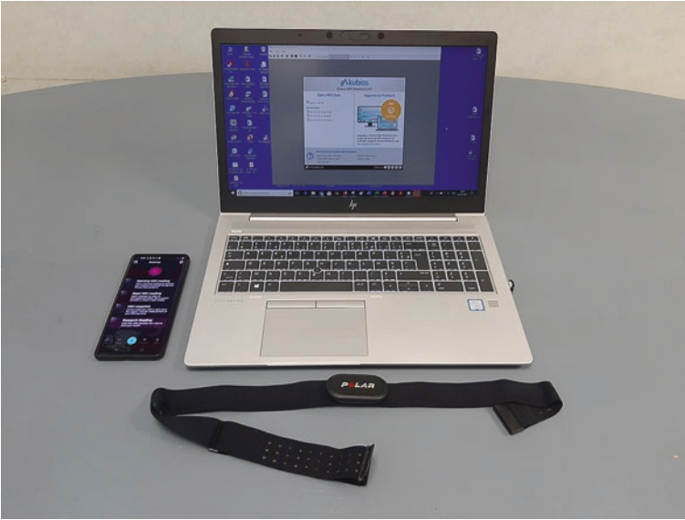
Fig. 5.3 Chest strap equipped with sensors. Signal transmitted to a memory buffer of a smartphone. Treatment on computer
